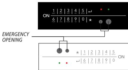
**After opening the lock, open the door within 10 seconds. If maximum time is exceeded, the door closes automatically**
